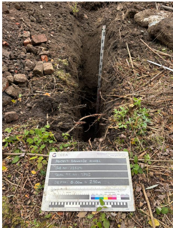
TP02 - Excavated to a depth of 2.90 m - looking north
