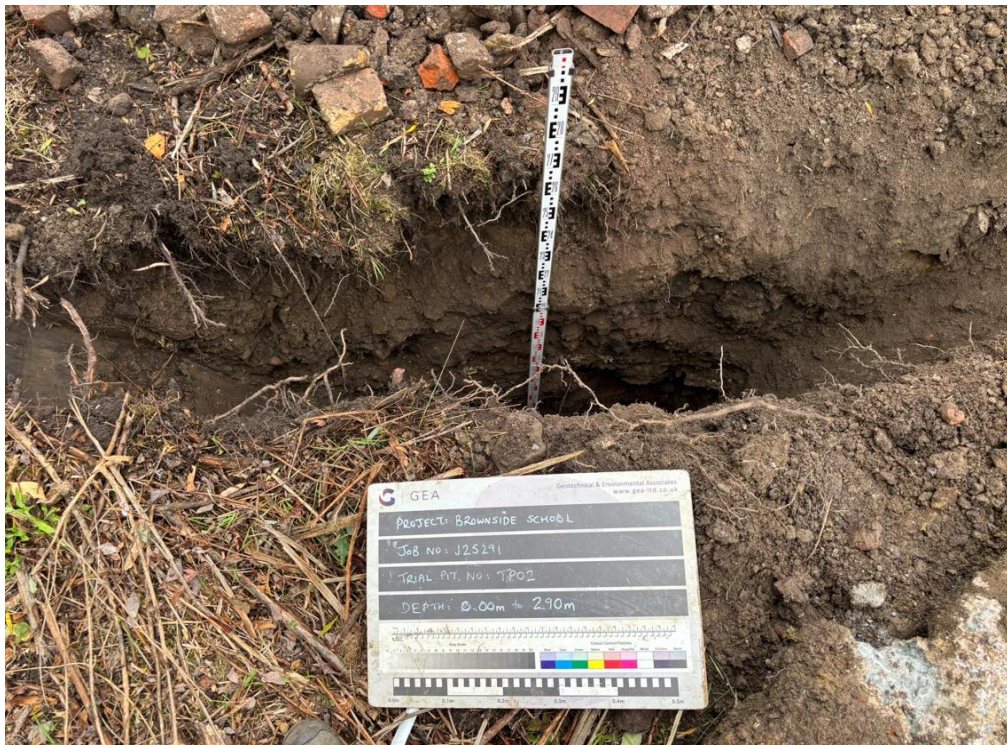
TP02 - Excavated to a depth of 2.90 m - looking west
