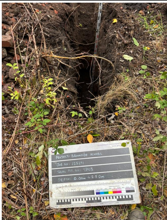
TP03 - Excavated to a depth of 2.50 m - looking north
