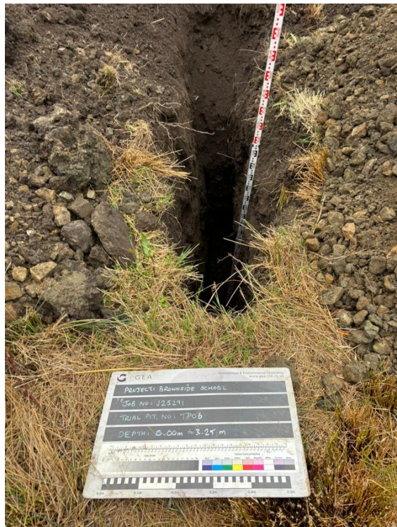
TP06 - Excavated to a depth of 3.25 m - looking north
