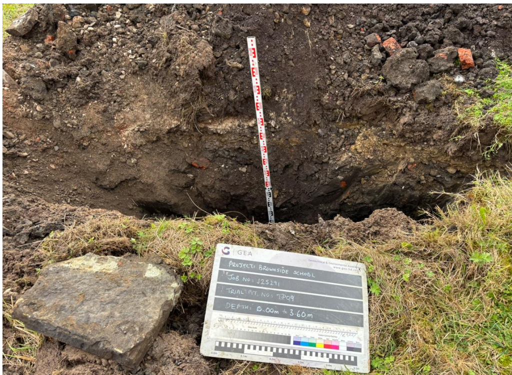
TP09 - Excavated to a depth of 3.60 m - looking west
