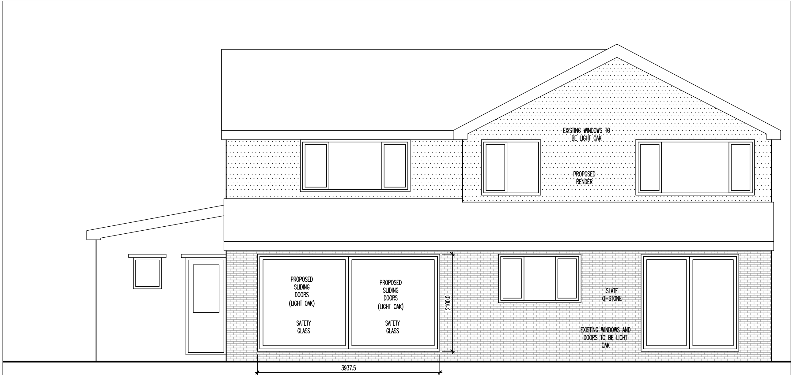
03 Proposed Rear Elevation Scale 1:50
