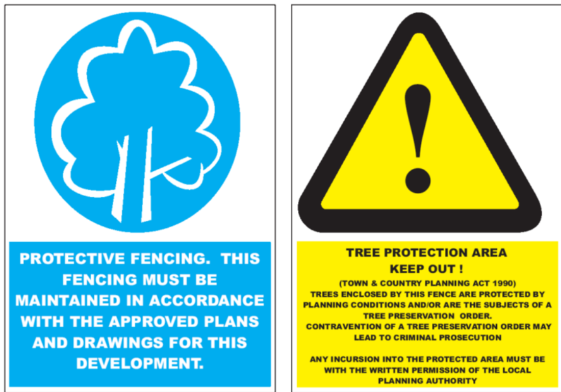
Figure 3: Example Tree Protection Area warning signs
