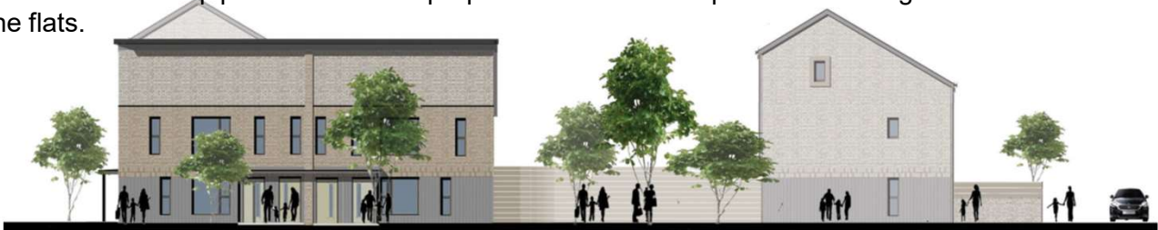
Elevation to flats with monopitch roof to maximise the noise reduction
