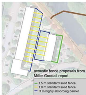
3000mm high fence: highly absorbing barrier
