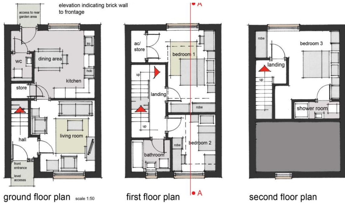
Figure 5 – Type C Terraced Houses Floor Plans
