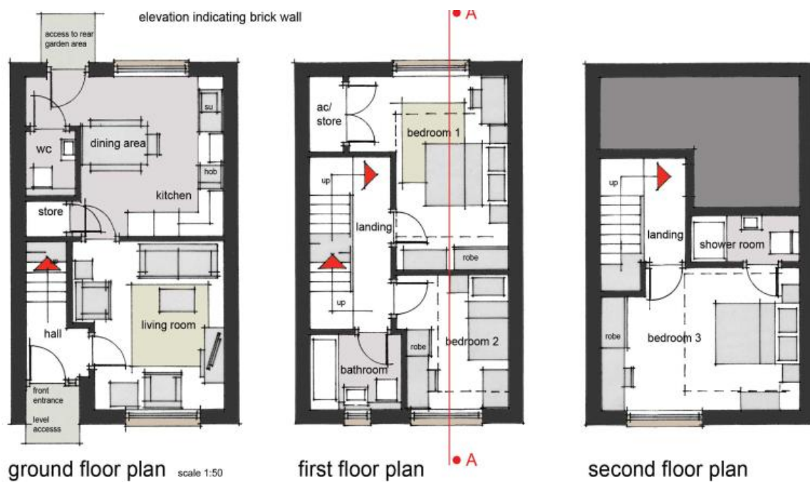
Figure 4 – Type B Terraced House Floor Plans
