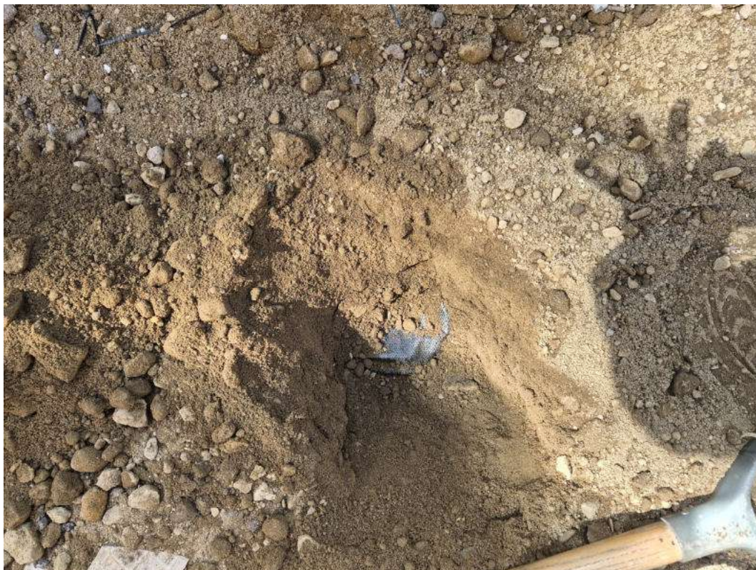
Photograph 18: Close up of validation pit 3. Geotextile barrier visible at the base – 6/5/2026.
