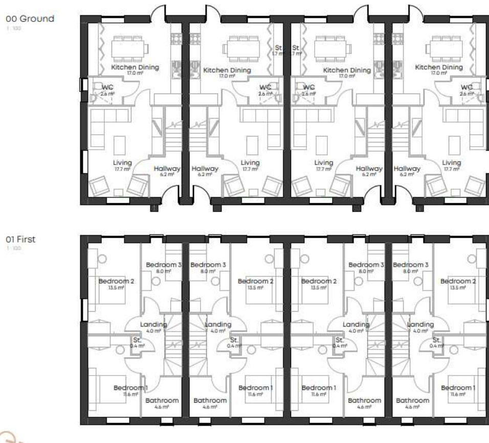
Figure 5 – House's Ground and First Floor Plans
