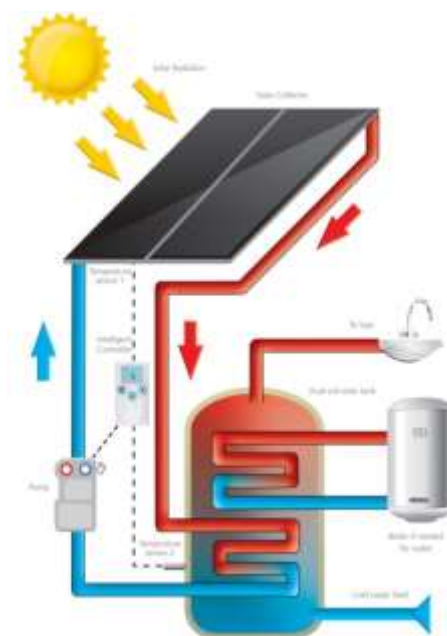
Figure 11 - The principles of a solar thermal system
