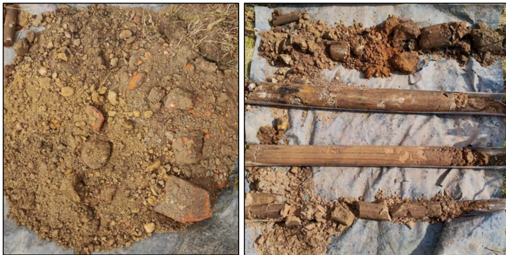
Figure 4: Photographs of the typical Made Ground (left) and Glaciofluvial Deposits (right) encountered.
