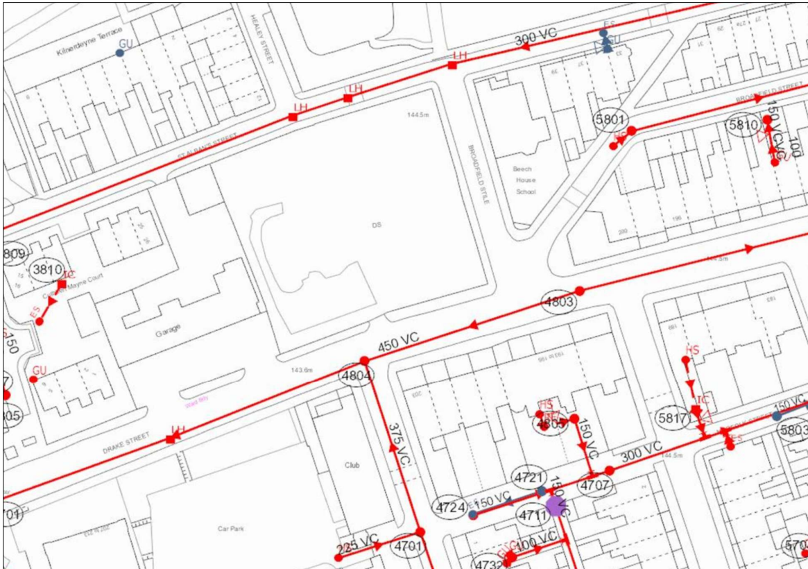
Figure 4.1 Excerpt of Water Authority Sewer Records (Source: United Utilities)
