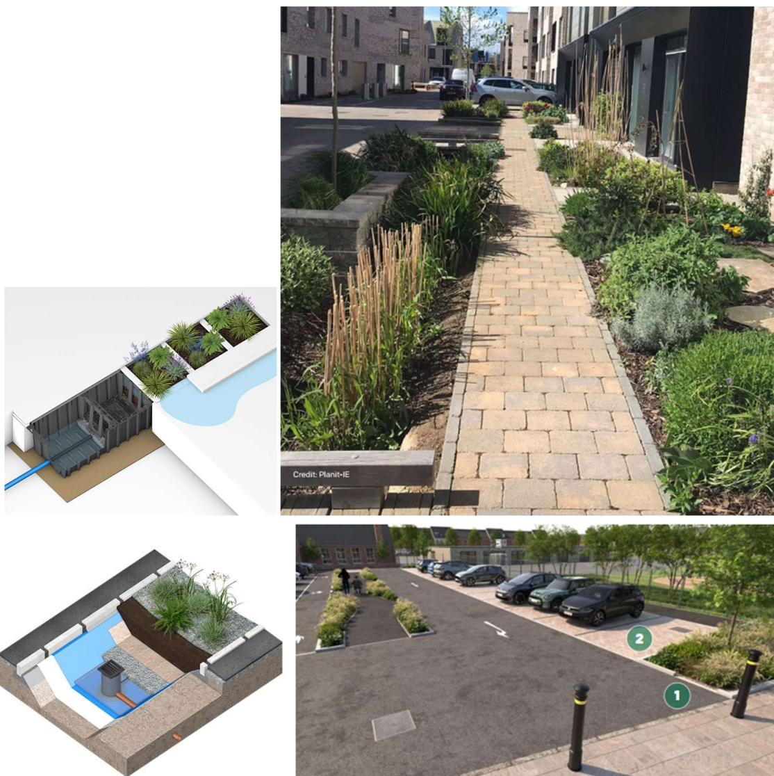
Figure 12.2 Bioretention / Rain Gardens / Hydroplanters
