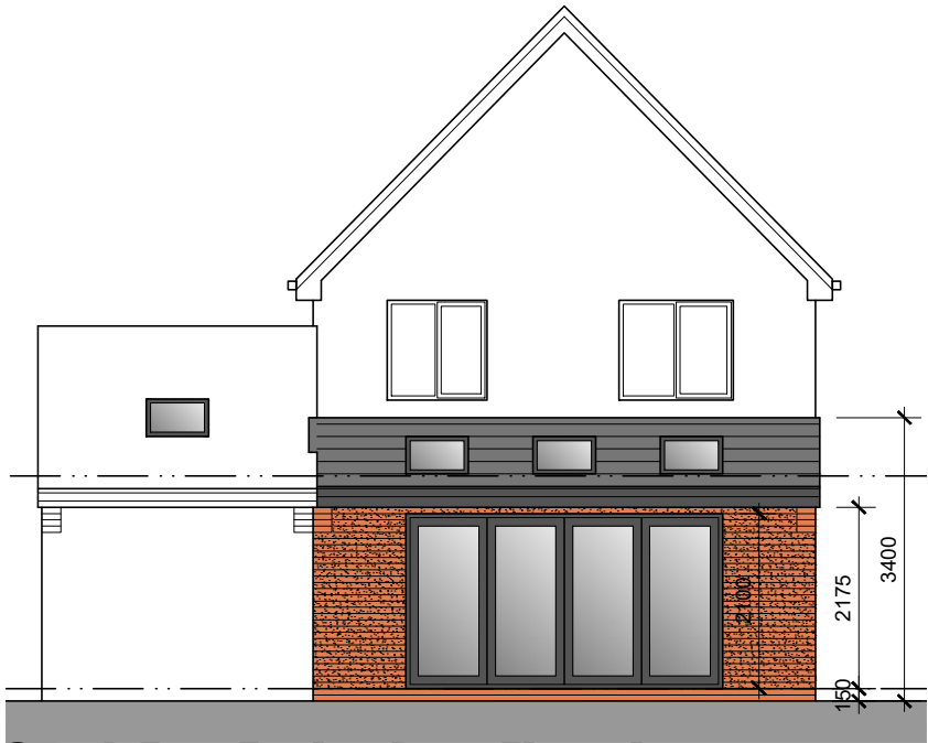
South East Facing Rear Elevation
