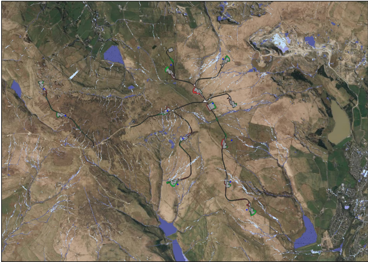
Figure 4-5 Surface Water Flooding with Scheme Overlay
