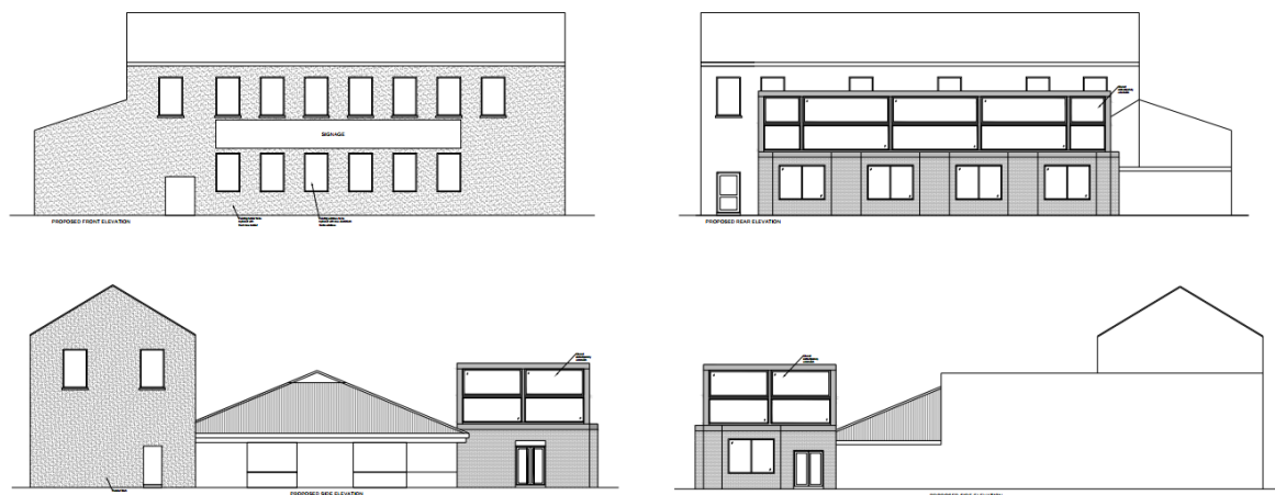
Figure 3: Existing/Proposed Rear Elevations Plan Extracts (NASA Design Studio), NTS
