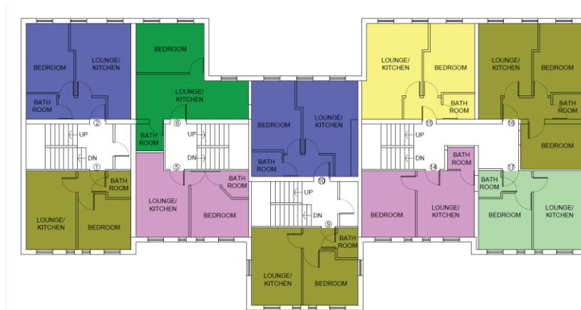
Figure 4 Original proposed layout of upper floor
