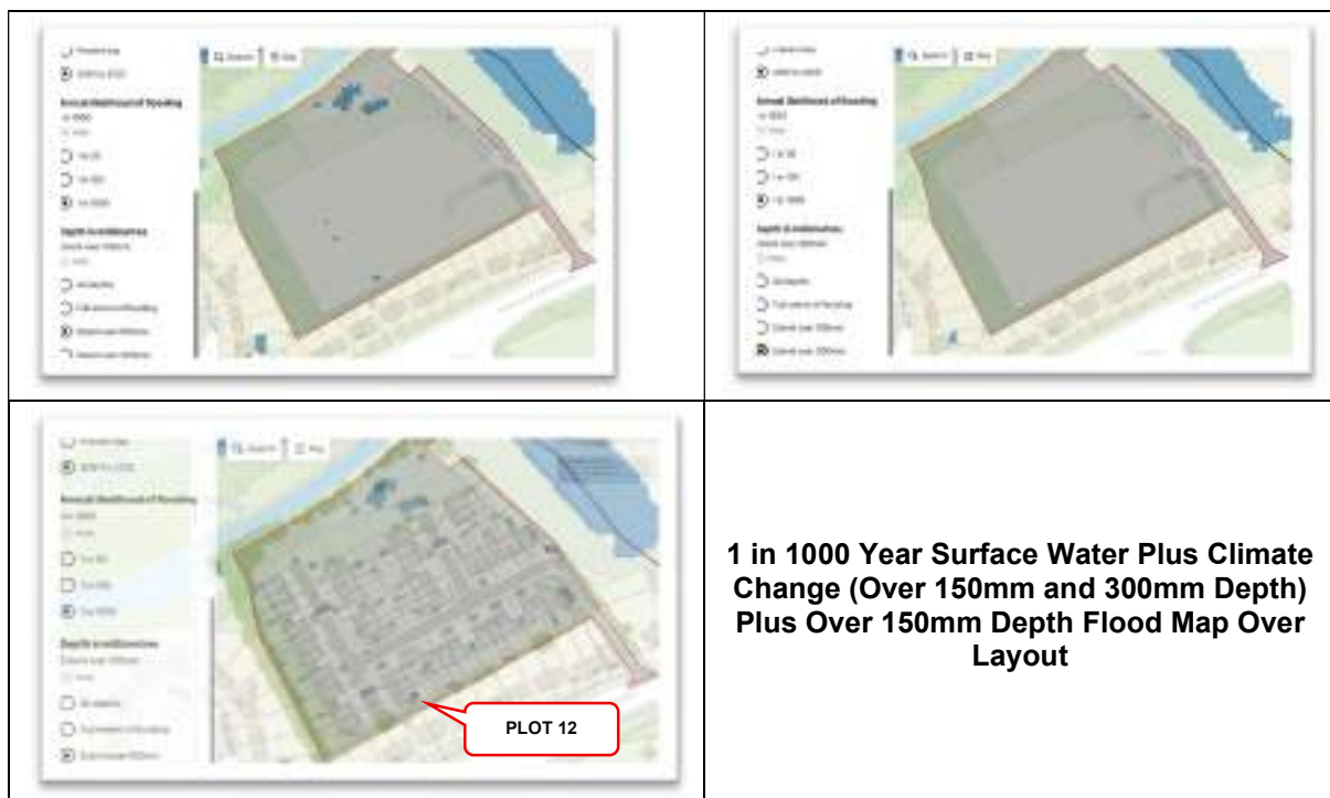
Figure 11: 1 in 1000 Year Surface Water Plus Climate Change (Over 150mm and 300mm Depth) Plus Over 150mm Depth Flood Map Over Layout
