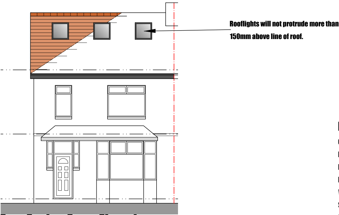
East Facing Front Elevation
