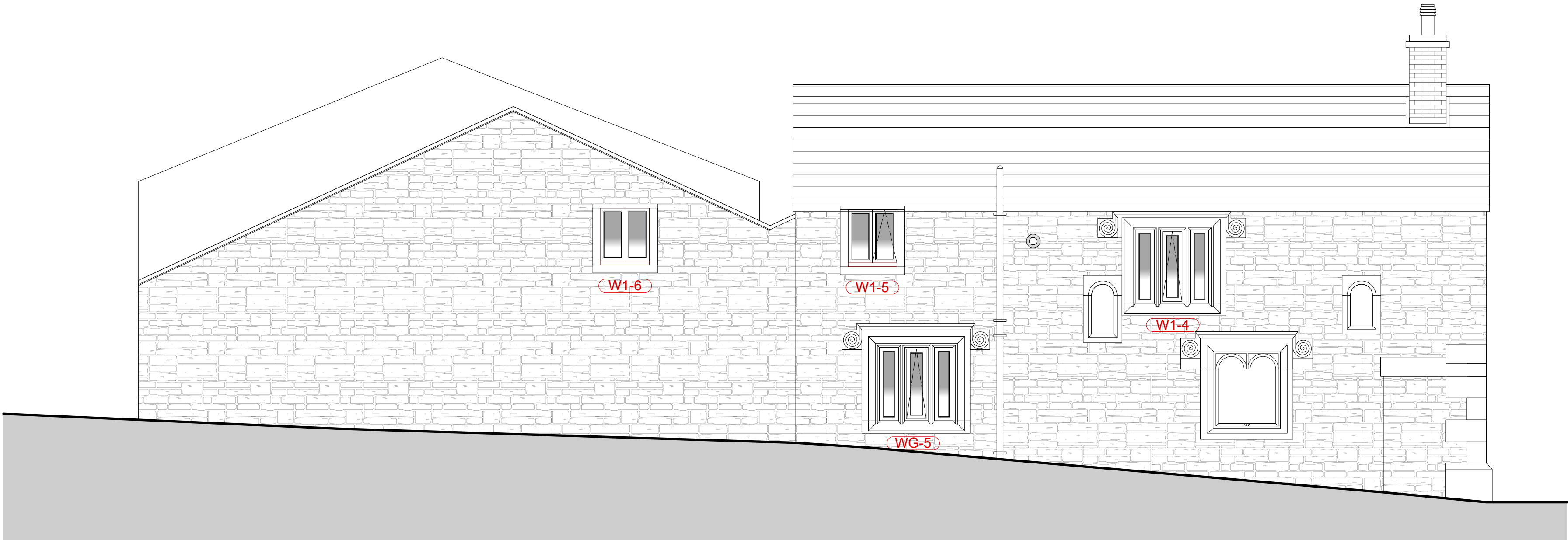
Proposed West Elevation Scale: 1:50
