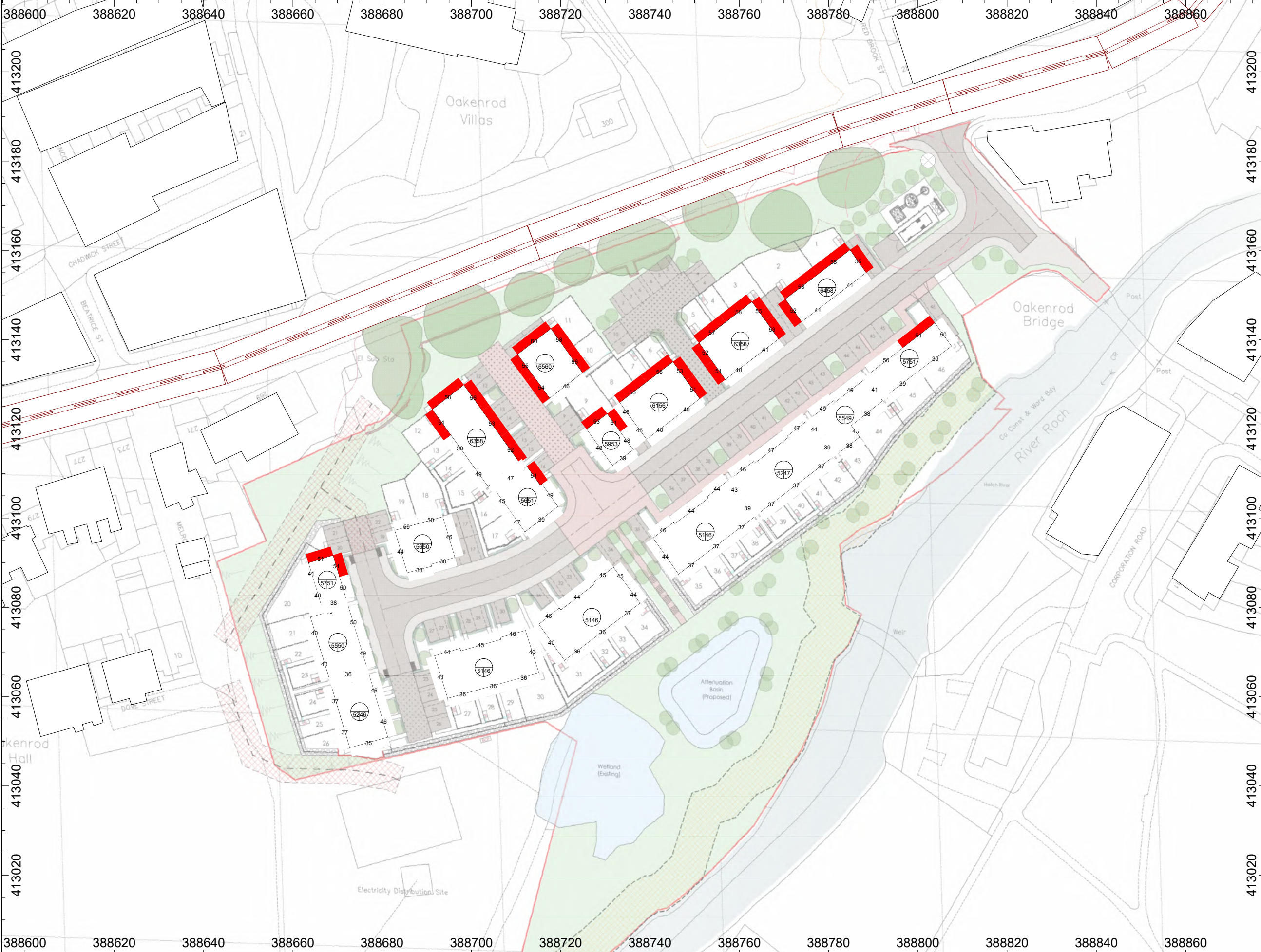
Figure 5 - Nighttime Overheating Risk Assessment - Calculation at 4.0m above ground level
