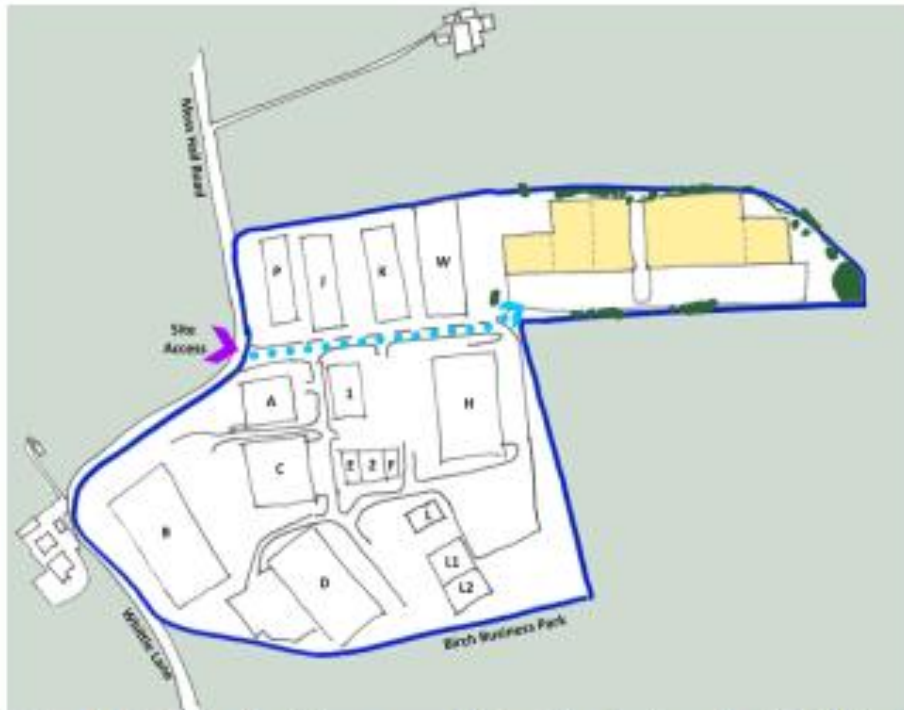
Option 4 - Revised option 2, in response to the existing terrain and reflecting the cut and fill exercise, the site is subdivided into two plateaus.
