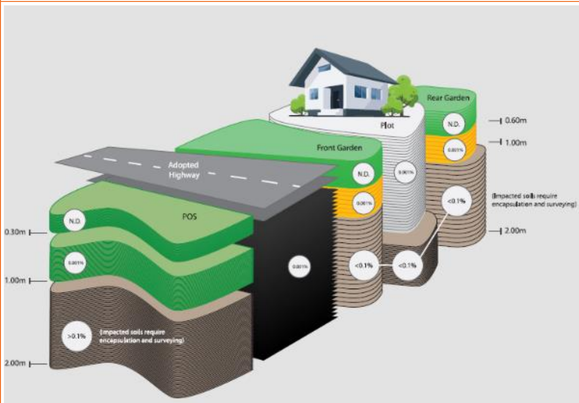
FIGURE 4.1 ASBESTOS RISK MITIGATION CONCEPTUAL SITE MODEL
