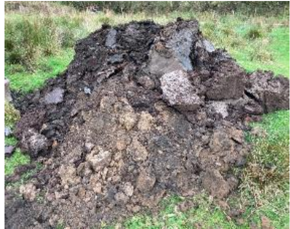
PLATE 9 TP115 EXCAVATION AND ARISINGS – NATURAL DRIFT WITH POCKETS OF PEAT
