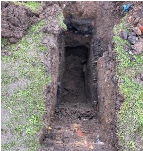
PLATE 8 TP107 EXCAVATION AND ARISING – MADE GROUND
