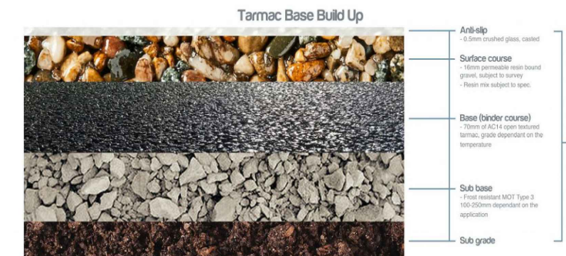
M1 - Driveway & Paths Surface Specialist Resin Bound Permeable Driveway (colour to applicants requirements) Permeable surface provides drainage
