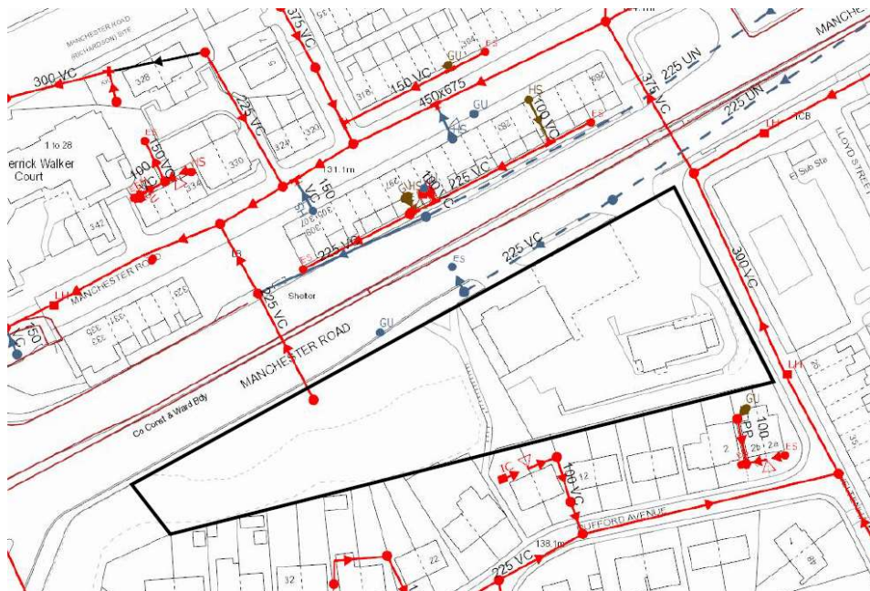
Figure 2.0 – Extract of United Utilities Sewer Record Plan
