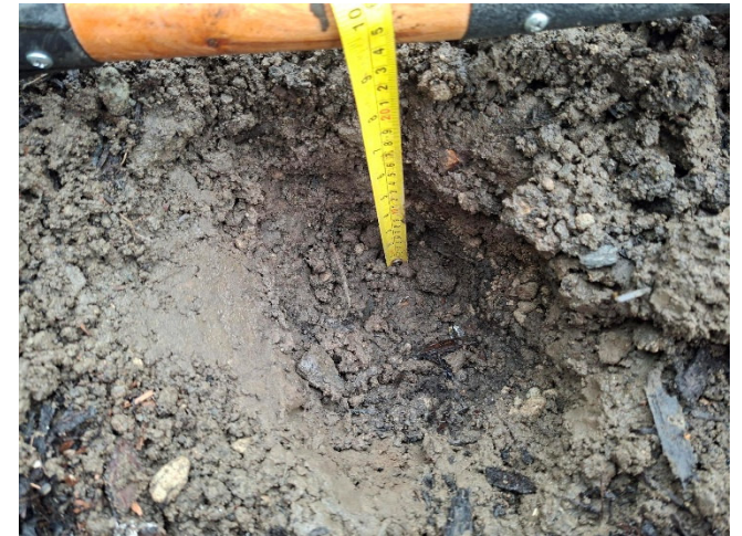
Image 12: Topsoil 3 location – woodchip / bark over topsoil
