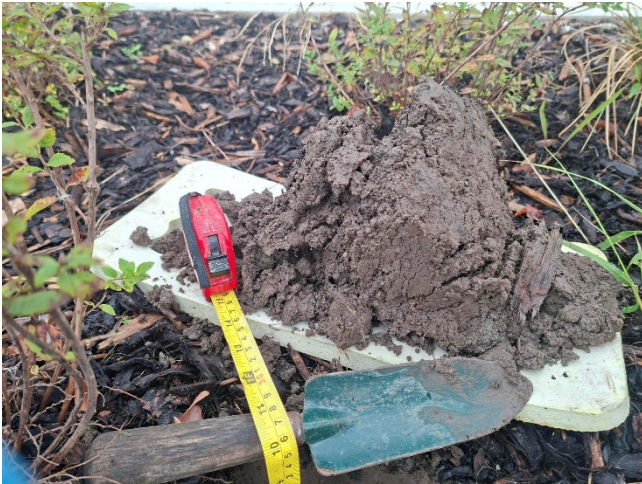
Image 10: Topsoil 2 location = 230mm depth
