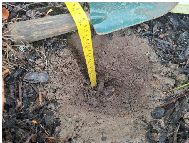
Image 5: Thin cover of bark over 230mm of brown sandy clay topsoil
