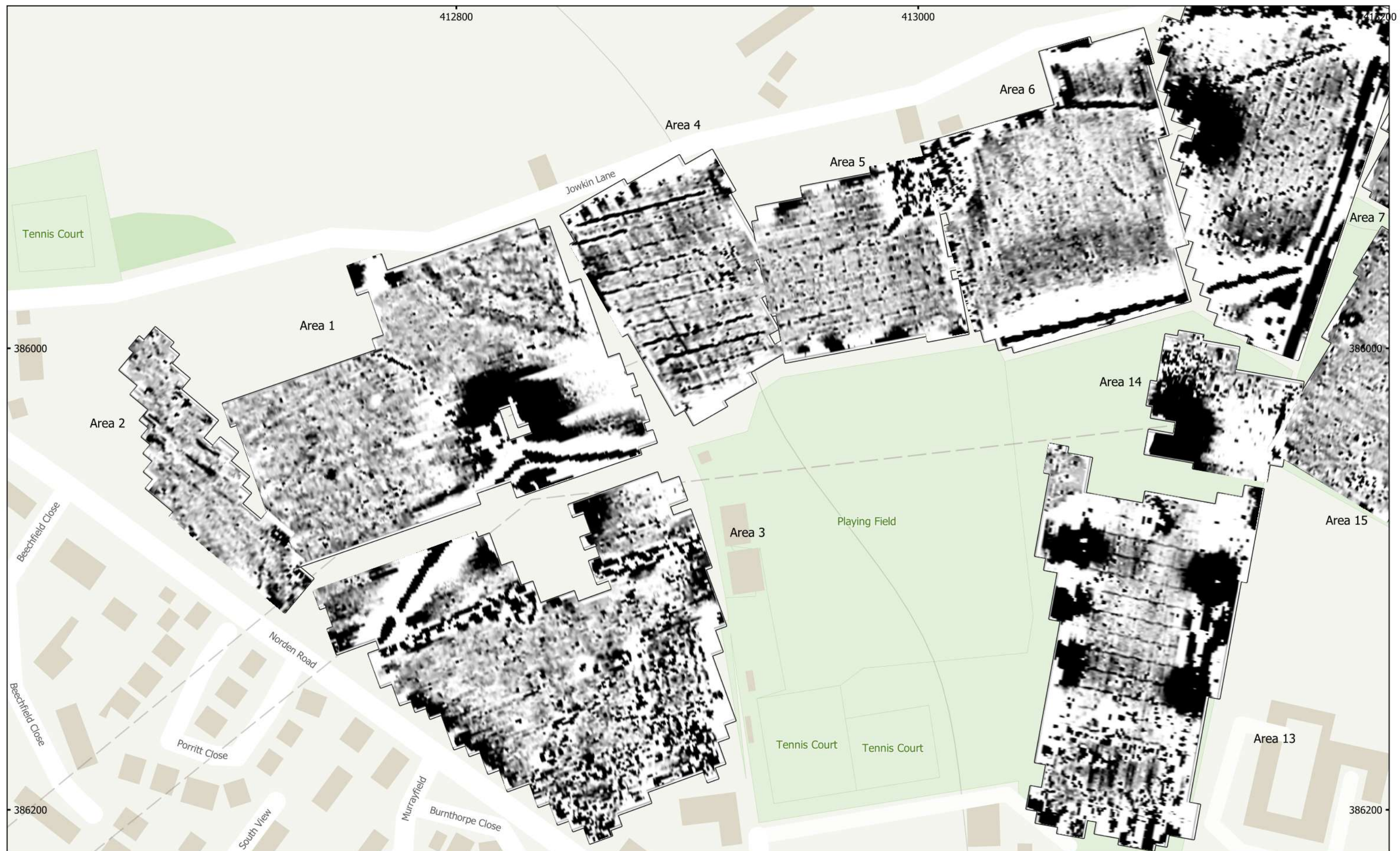
MSSD1116 - Bamford, Norder, Rochdale Figure 11 - Magnetic Gradient (Area 1, 2, 3, 4, 5, 6, 7, 13, 14 & 15) 1:1,500 @ A3 Copyright Magnitude Surveys Ltd 2022 Contains Ordnance Survey data © Crown Copyright and database right 2022
