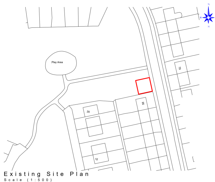
Figure 4: Existing site plan (extract from drawing 002 - C200-356, 1:500). Red line site area approx. 70.34 sq m (0.007 ha), about 3.5% of the 0.2 ha Regulation 7A threshold.
